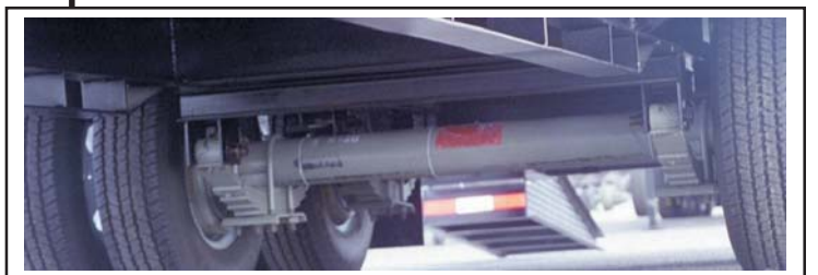
Dexter axles with 3" heavy duty rubber bushed suspension
